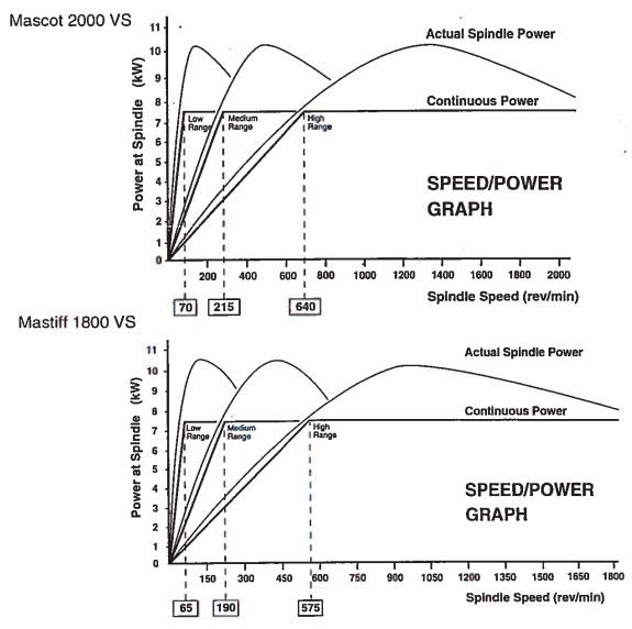
Example of spindle speed calculation.
