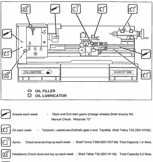
Gearbox. Check level and top up each week - Shell Tellus T32 (ISO HV 32). Total Capacity 2.8 litres.
