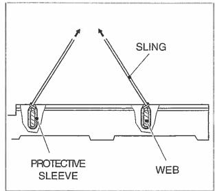
5. Carefully lift the lathe clear of ground and if necessary reposition slings to achieve balance before lifting further.
